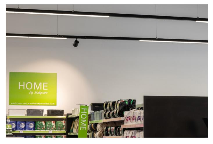
The E-Line LED continuous line system, known for its groundbreaking light quality, proved the perfect solution for stores without a ceiling grid. This system offers the flexibility to add spotlights to highlight specific product displays in suspended versions. The choice of black fittings helps the luminaires fade into the background, allowing the lighting distribution to guide and entice shoppers.
