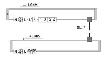
Connection of sensor units to controller luminaires is as described above. A maximum of two sensor units can be connected in parallel via an OMD2 two-way distributor. Correct addressing of the sensors must be ensured here, as described in the sensor settings section. The table on page 39 specifies technical data for the sensor connection.
