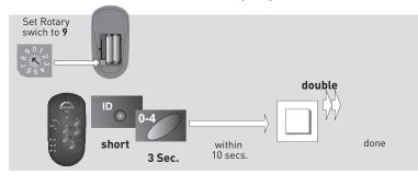
Up to 5 different addresses (0-4) can be assigned. The factory presetting is address 1.
