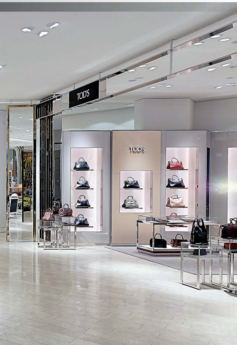
The lighting planners arranged the Cardan series spotlights into triangles to create the illusion of halos on the product display tables.
