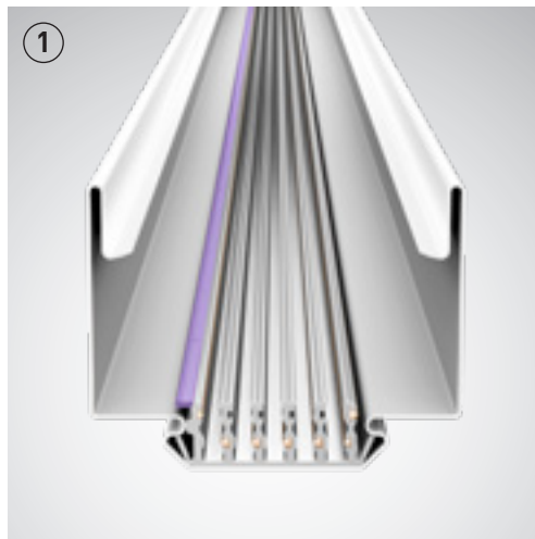
7-core current conducting profile 5 \times 2.5 \text{ mm}^2 + 2 \times 1.5 \text{ mm}^2 3 separate circuits 2 control lines for DALI signal
