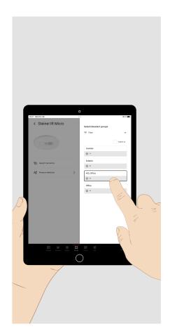
In this menu, the **functions** of the sensor can be called up and assigned to **one or more luminaire groups**.
