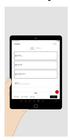
If a light scene is set as the default light scene, it is called up after switching on the mains supply to the lighting.
