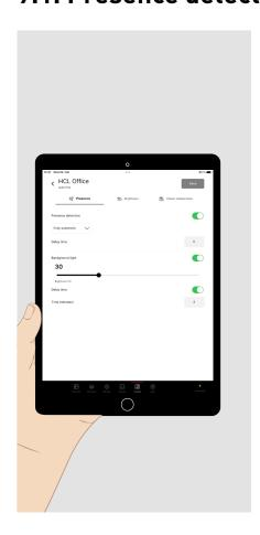
When parameterising a group in a light scene, functions for presence detection, brightness control and (with Tunable White luminaires) colour temperature control can be set.
