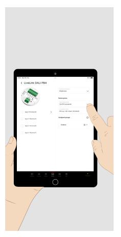
In this menu, the functions of the push-buttons of a push-button coupler can be called up and assigned to one or more luminaire groups or scenes.
