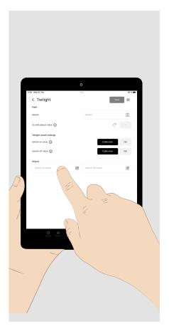
Set up a twilight switch to automate switching on the lighting when it gets dark and switching it off when daylight comes.
