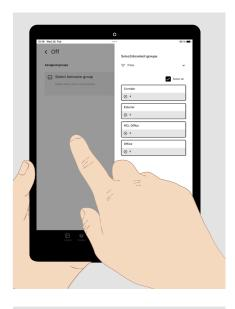
If several luminaire groups are to behave identically in a light scene, the parameterisation of one group can be transferred to other luminaire groups. An example of such a scene can be a central **Off function**.
