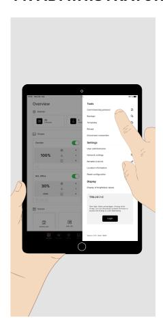
If you logged in as "administrator", the necessary steps for commissioning are also available. For these, tap "Structure", "Devices", "Groups" or "Scenes" at the bottom of the screen. The main menu called up is shown in a light-coloured font and with a red indicator bar (see the following section).
