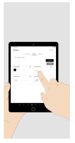
In the "Sensors" submenu of the "Groups" main menu, the functions of the sensors can be assigned to the created luminaire groups.
