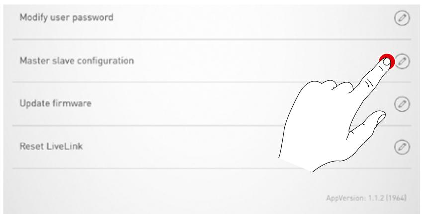
First all slave control units must be configured with the slave operating mode
