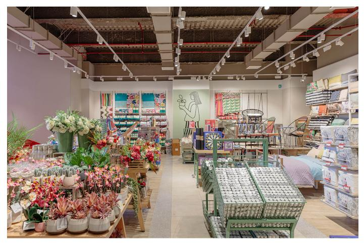
The store design is based on open structures with fluid transitions between areas. To visually reinforce this approach, TRILUX used a mix of suspended track lights, recessed spotlights, linear lighting systems, and discreetly integrated wall washers. The goal was to create a homogeneous yet differentiated lighting scheme that accentuates textures, colors, and materials.
