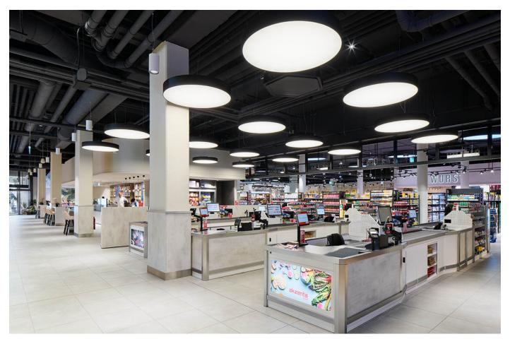
Power tracks also serve as the basis for the frozen goods, where they are fitted with Lightpanels in the cooler 4000 Kelvin light color to match the product range. Finally, the long-distance effect of the large, round Loretto pendant luminaires above the checkout area cleverly directs customers to the checkout.
