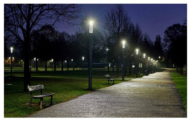
Thus, the entire outdoor area was illuminated with the ConStela 19 LED. This smart solution, equipped with the optical MLT system (Multi Lens Technology System), enables extremely flexible and precise adjustment of the light distribution to the general conditions on site, creating perfectly illuminated paths and squares.
